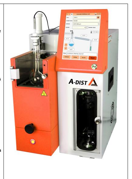
**A-DIST: Test principle** During the test, the sample is placed in a distillation flask and distilled exactly according to the conditions specified in the standards. The sample is heated and the generated steam is cooled in the condenser and collected in a graduated cylinder. All results, both analysis and timing, are automatically recorded during the test.
